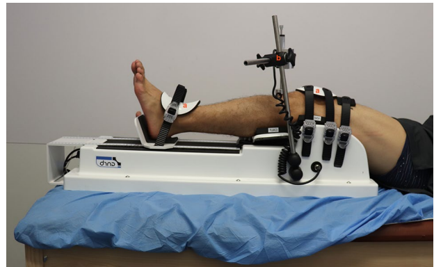
Fig. 2 The GNRB measurement set-up. All straps were securely fastened (a), the sensor was placed perpendicular to the tibia (b) and the sequence was run
